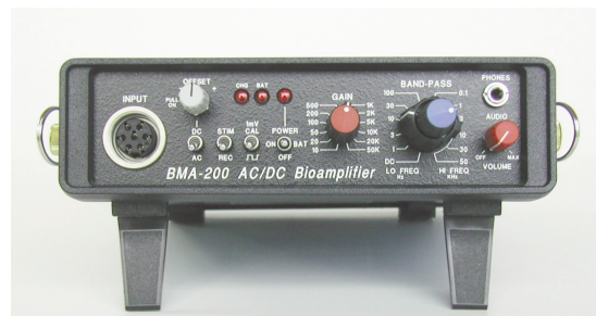
BMA-200 single channel, portable preamplifier
