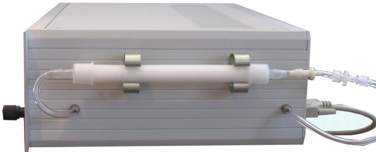
Figure 3: Side view of MM-100 showing desiccant tube. Note required in-line filter to the right.
