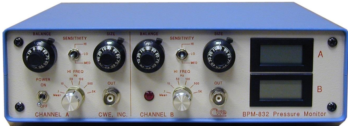
Figure 1: Front panel view of BPM-832, showing the two identical sets of controls.
