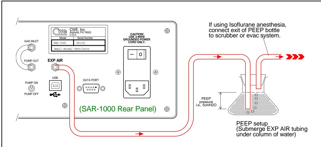
PEEP setup using SAR-1000 ventilator
