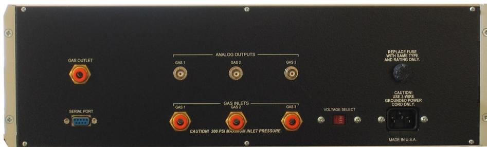
Rear-panel view of the GSM-3 Gas Mixer, showing the three gas inlet connections and the mixture outlet to the left (1/4" quick push/pull connectors). The three BNC jacks provide an analog voltage corresponding to the concentration of each input gas in the programmed mixture.
